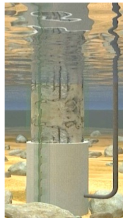
Step: 4 Connect hose and pump 500mm plug, let the plug cure
